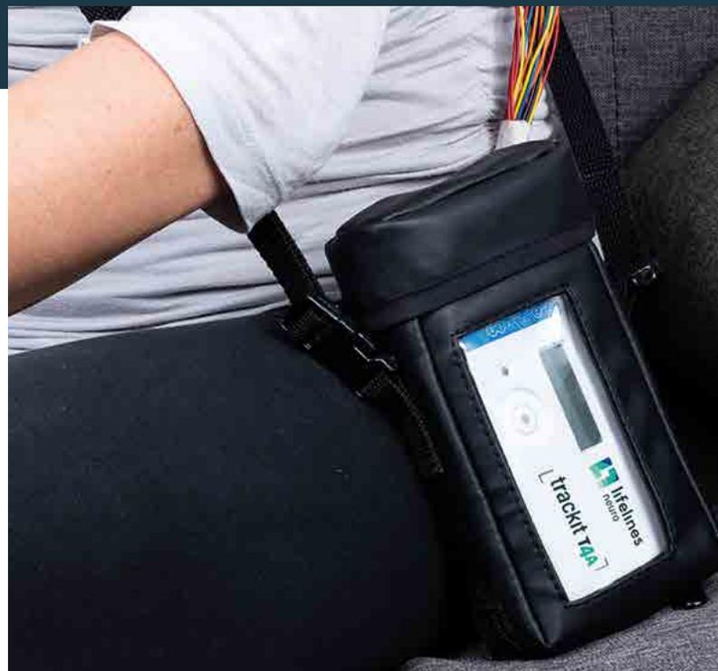
Trackit T4A is a high performance ambulatory EEG recorder for use with Lifelines Neuro's ambulatory systems. It is a low power, battery-operated recorder, with 28 monopolar and 4 user configurable channels, delivering the highest quality EEG for up to 72 hours continuously using Trackit and Trackit Plus software. Data can be read anywhere, anytime using dedicated cloud software.
