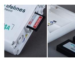
While the energy efficiency of the T4A enables it to run for 72 hours on two rechargeable batteries, high volume practices will want to ensure a ready supply of charged batteries is on hand. This is valuable for back-to-back studies or for those studies that need to be extended. Techs can simply swap fresh batteries, SD card, and electrodes in minutes.
