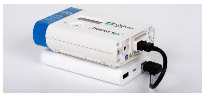
c. Place the External Power Bank and T4A inside the pouch. Electrodes can be plugged in before or after placing the T4A in the pouch. Most find it easier to plug them in before.
