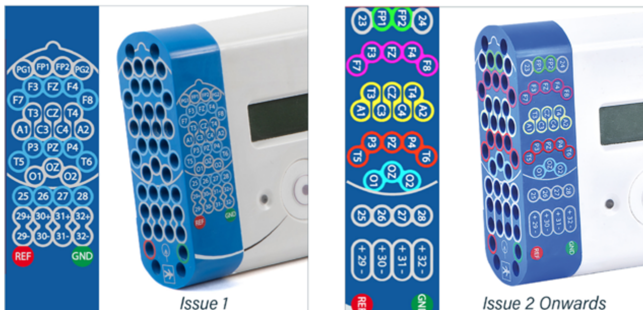
Figure 5: Connecting the Trackit T4A Amplifier (PCU/front face)
