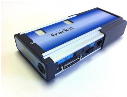
Figure 46 Trackit Mk3 with Internal Bluetooth Module
