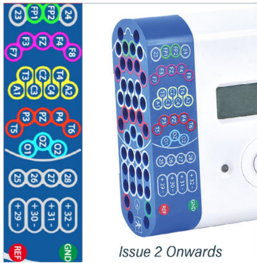
Figure 5: Connecting the Trackit T4A (PCU/front face)
